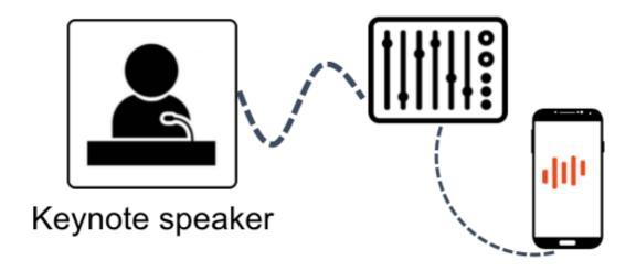
Of course, you can also use a smartphone for the transmission of original audio via a mixing console. Since smartphones will recognize an audio input only if you use a 4 pole plug, you might need an adapter from 3 to 4 poles, like this one, which you get for a few Dollars.
