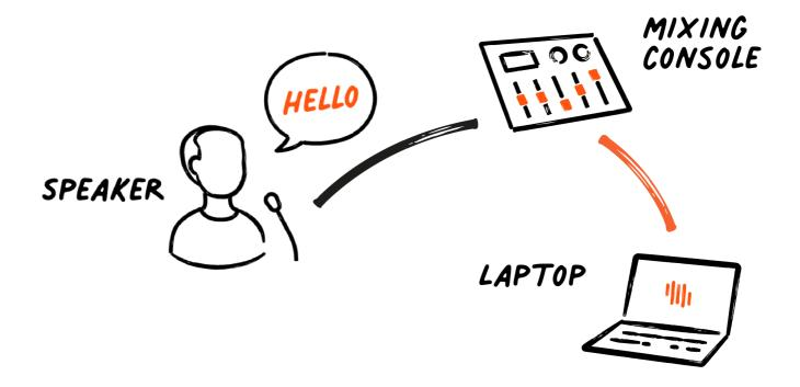
If you want to stream the original audio from stage, the most common way will be to get your signal from an audio mixer into your laptop or PC. You usually do this with an USB audio interface, like this one.
